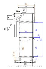
Electrical inlet (power) ΕI Refrigerant Inlet RO Refrigerant Outlet
